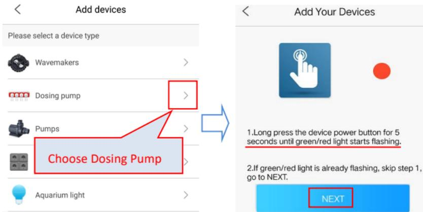
Before connecting your pump to Wi-Fi, please make sure your pump is on connection status – the Wi-Fi Indication Light is flashing in green and red. Press the Wi-Fi button for 10 seconds to reset the Wi-Fi. All previous network information will be deleted.
