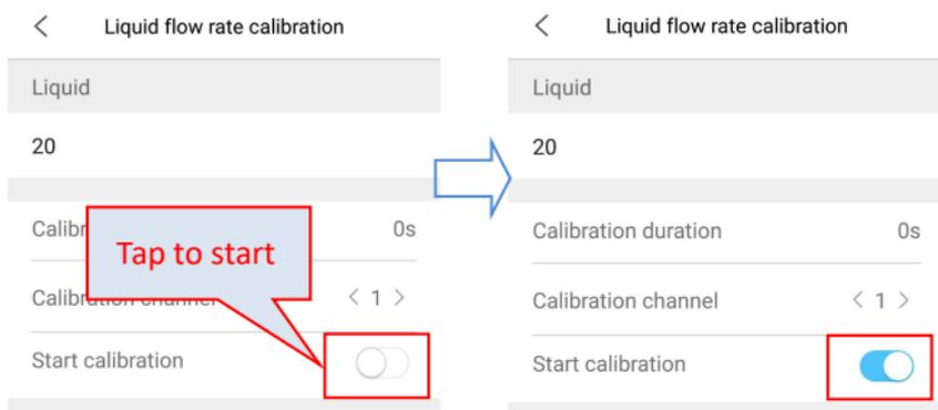
When the cylinder liquid is 20ml, tap the “Start calibration” switch to be off, then the channel 1 calibration stops.
