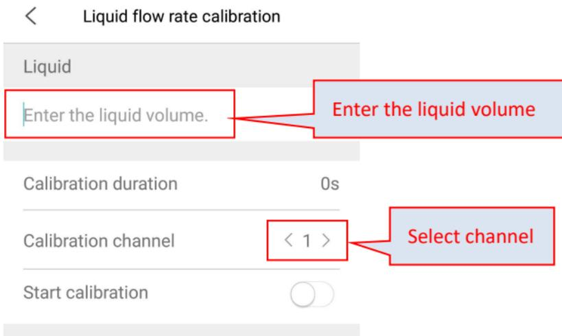
**NOTE:** For increasing the dosing precision, please refer to the actual dosing liquid volume for calibration. The calibration liquid volumes can be set to 10,20,30,40,50,60,70,80,90,100 (ml), and the calibration duration will be stored in the memory. The closer the calibration volume is to the actual dosing liquid volume, the more accurate the actual dosing liquid volume will be.
