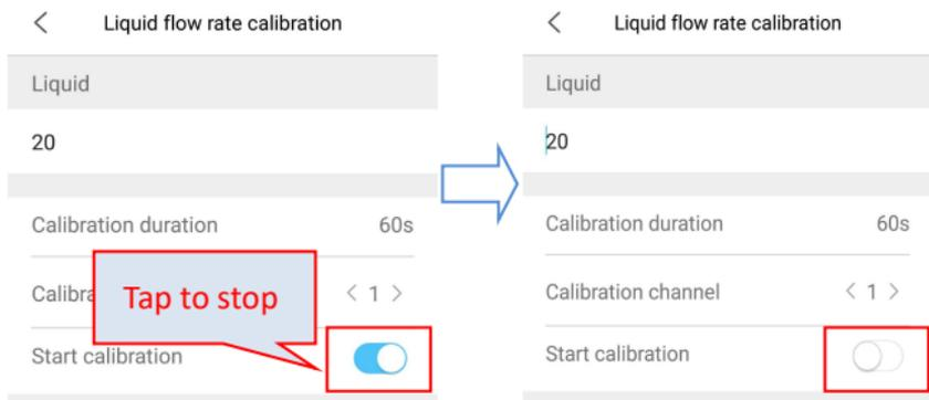
The calibration duration is shown. And the channel 1 calibration completes.
